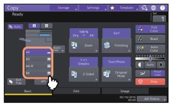
When using bypass copying, be sure to set the paper size. For instructions, refer to the *Paper Preparation Guide*.
