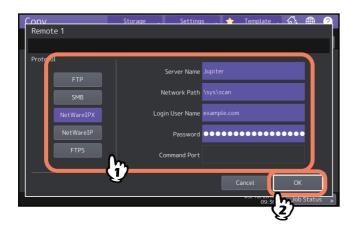
When you press any of the buttons below, the on-screen keyboard appears. When you finish the entry, press [OK].
